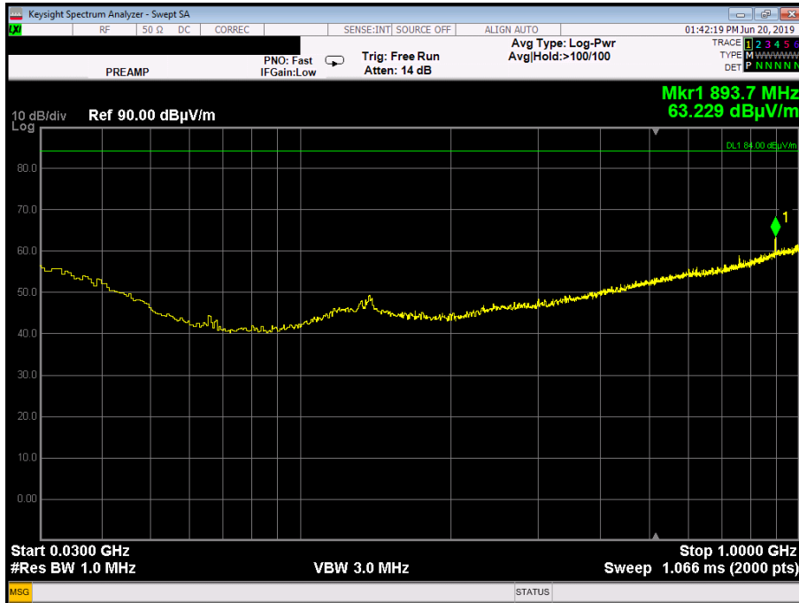
Plot 3.6.10: Spurious Emissions test results, 30 MHz – 1GHz range, Vertical polarization, High Frequency
