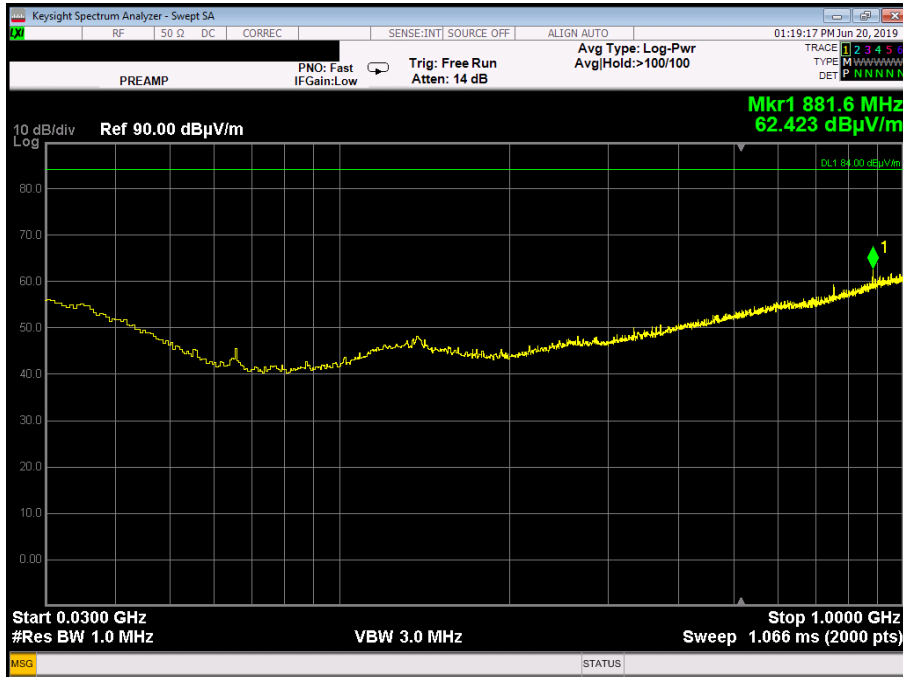
Plot 3.6.6: Spurious Emissions test results, 30 MHz – 1 GHz range, Vertical polarization, Middle Frequency
