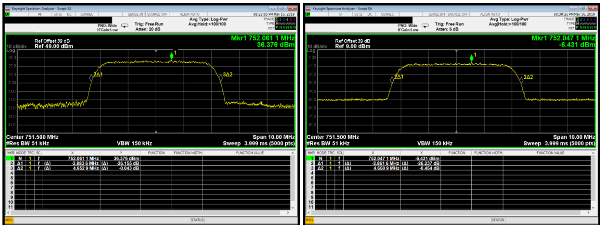
Plot 3.2.2: Input-versus-output signal comparison, AWGN 4.1MHz, 3 dB above AGC threshold level
