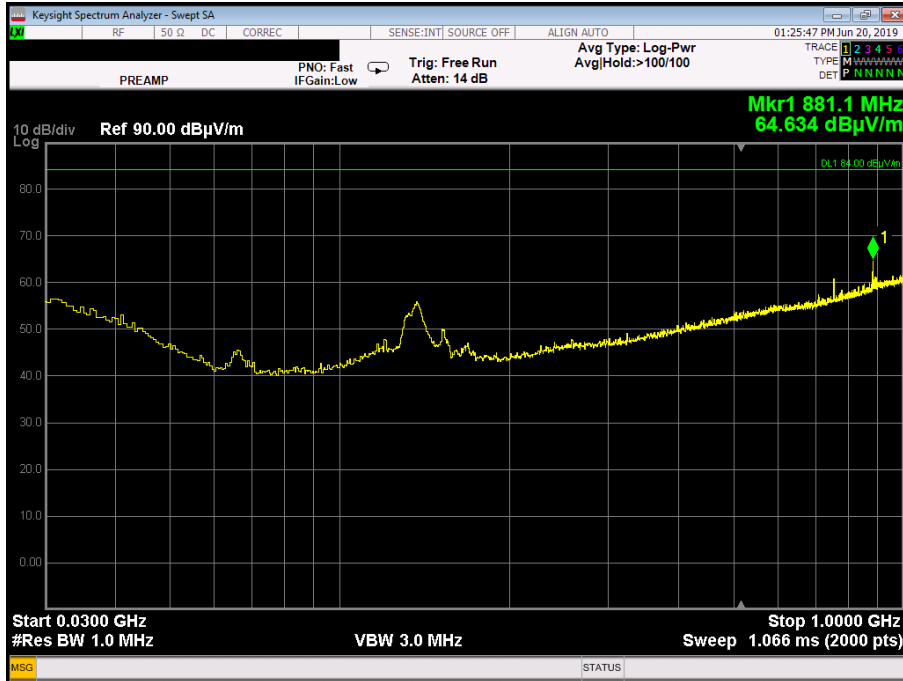
Plot 3.6.5: Spurious Emissions test results, 30 MHz – 1 GHz range, Horizontal polarization, Middle Frequency
