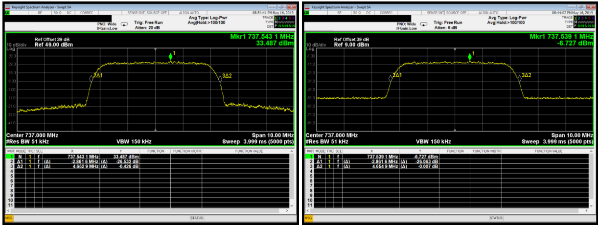
Plot 3.2.1: Input-versus-output signal comparison, AWGN 4.1MHz, 0.5 dB below AGC threshold level
