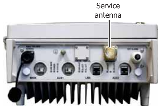
Figure 5-30. Front Panel Example showing Antenna Connection Port
