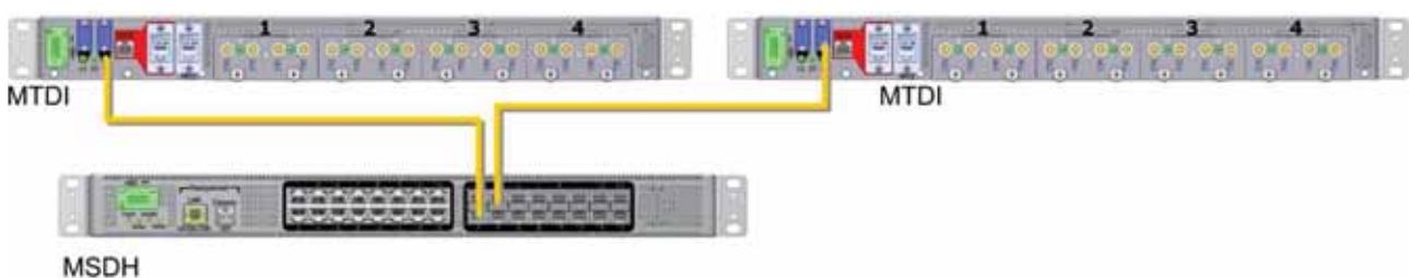
Figure 4-7. Example of MSDH to MTDI Connections
