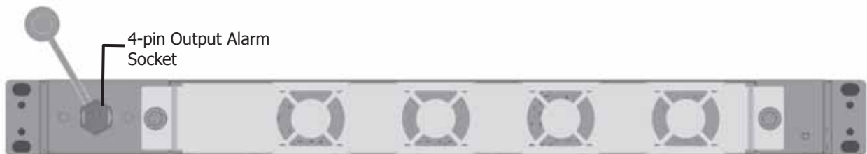
Figure 4-9 MSDH Public Safety Output Alarm Connections
