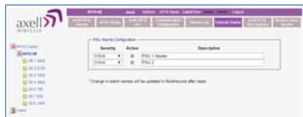
Figure 6-33. External Alarms Definitions
