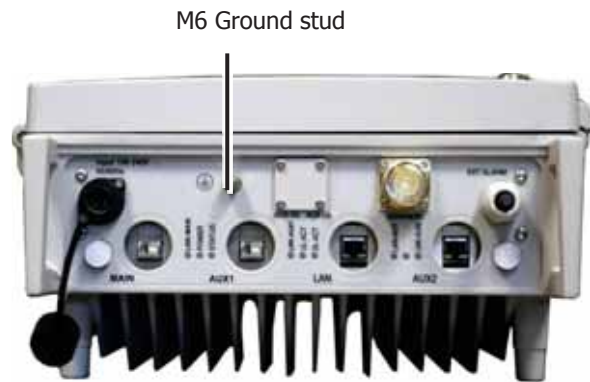
Figure 5-23. Grounding the idRU
