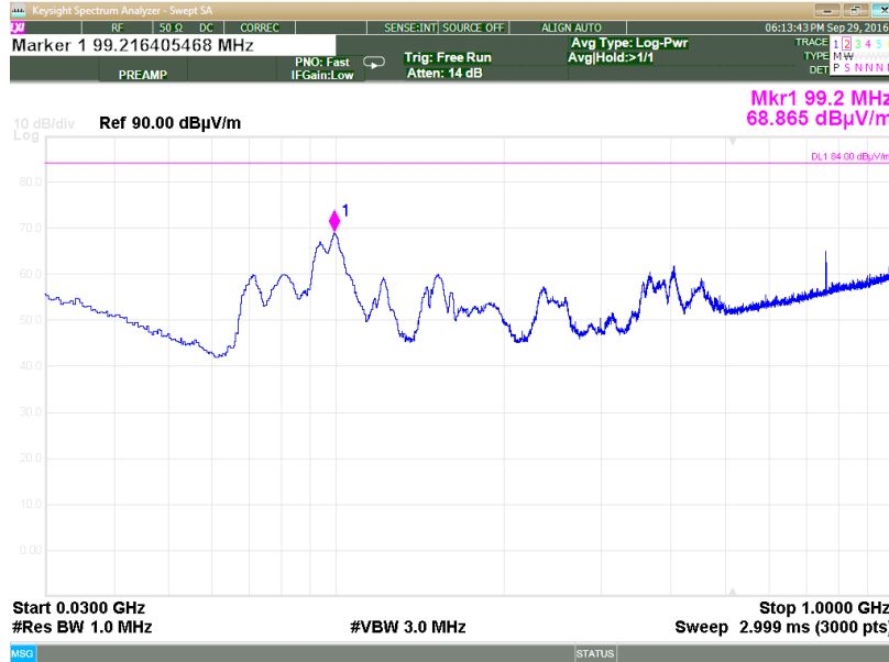
Plot 3.6.22: Spurious Emissions test results, 30 MHz – 1 GHz range, Vertical polarization, High Frequency
