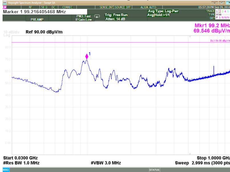
Plot 3.6.17: Spurious Emissions test results, 30 MHz – 1 GHz range, Horizontal polarization, Middle Frequency
