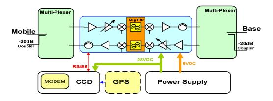
Figure 1: DMBR Simplified Block Diagram
