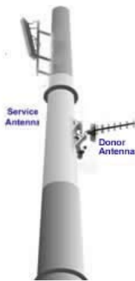
Figure 3. Service above Donor Antenna
