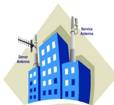
Figure 6. Service and Donor Antennas Installed on Opposite Sides of the Building
