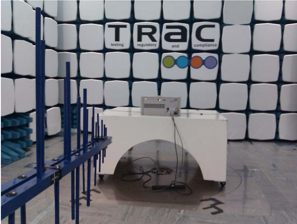
Photograph 1: Radiated test setup
