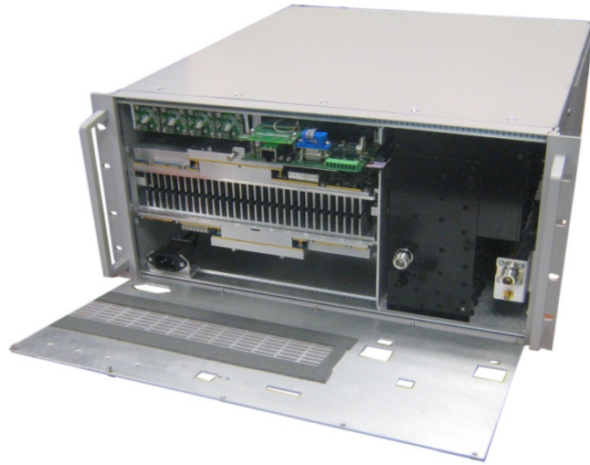
Figure 3. D-MBR with Removed Front Panel
