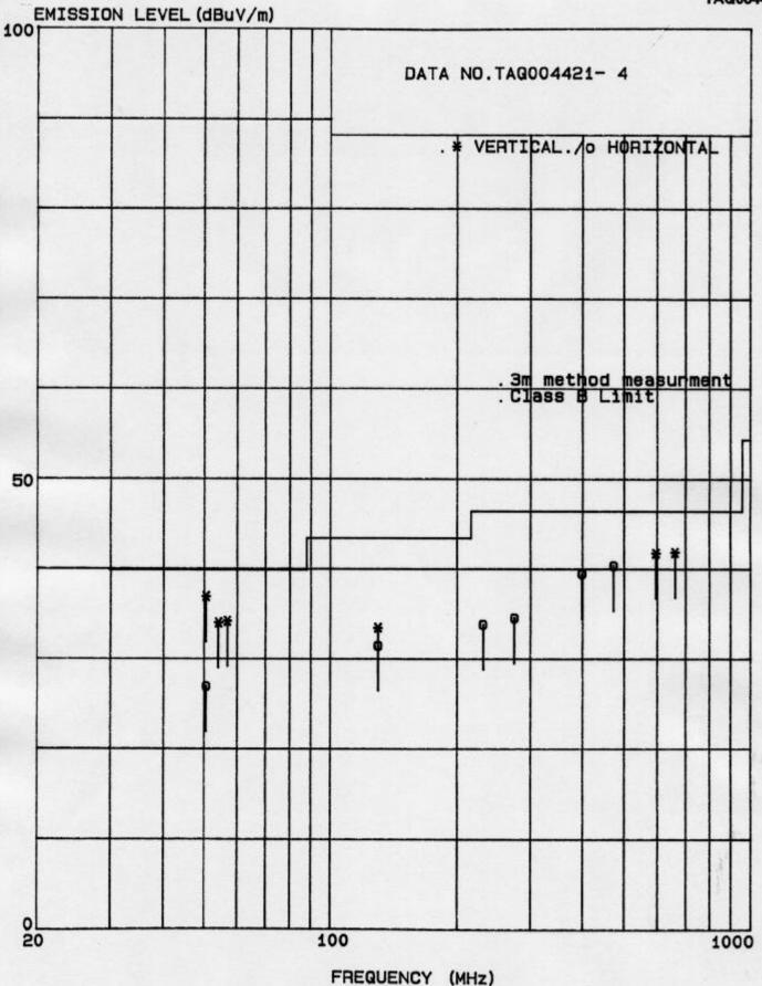
Figure 6.2-2 RFI Field Strength Measurement Results
