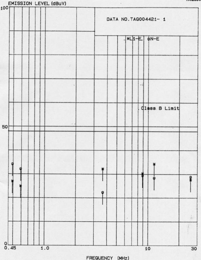
Figure 6.1-1 RFI Voltage Measurement Results
