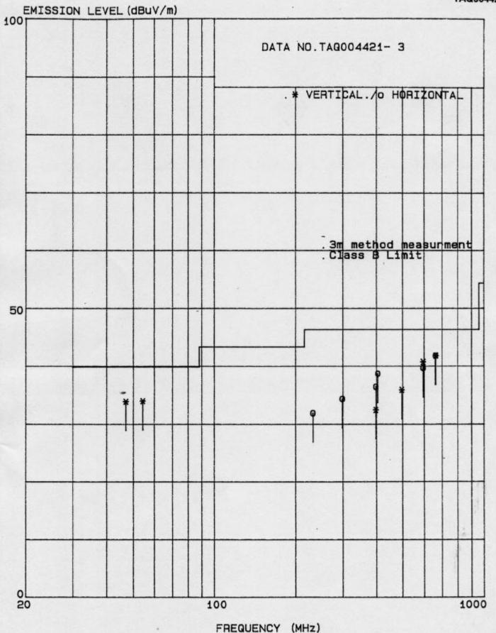
Figure 6.2-1 RFI Field Strength Measurement Results
