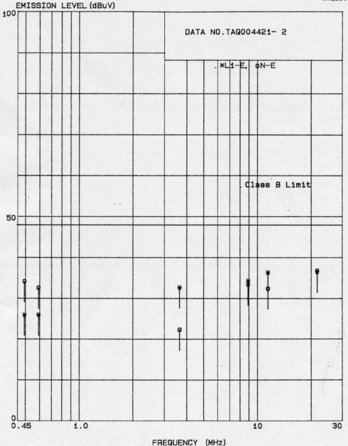
Figure 6.1-2 RFI Voltage Measurement Results
