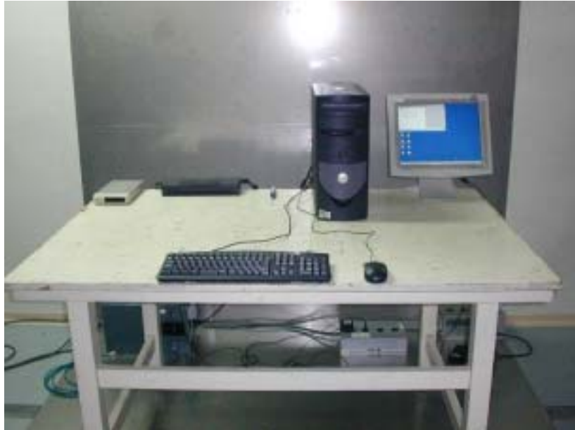
Photo 7.1a Setup with the Maximized RFI Voltage Emission Level < Communication mode >
