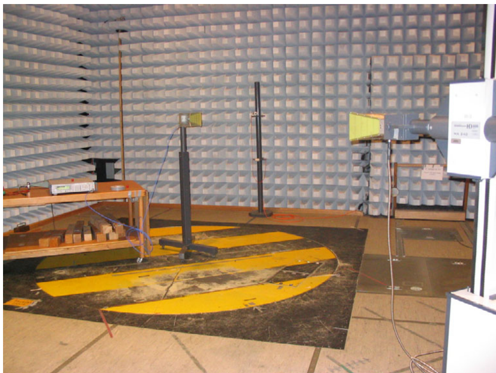
Fig. 29 – Photograph of the anechoic chamber with the test configuration for substitution method
