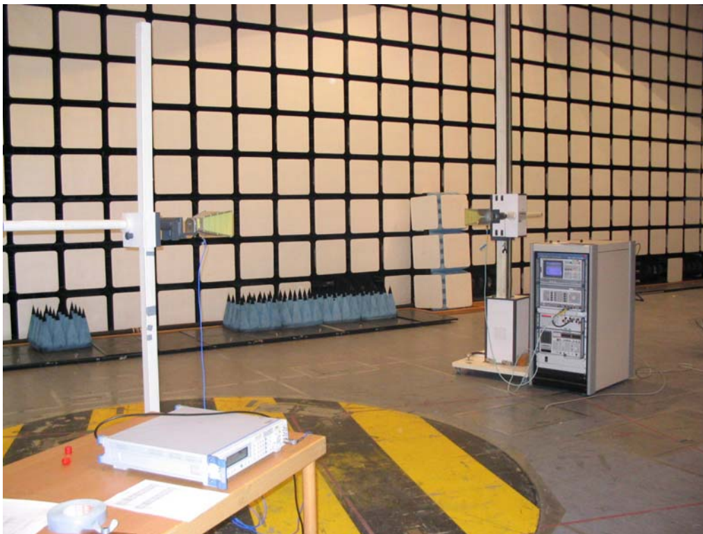
Fig. 68 – Photograph of the anechoic chamber with the test configuration for substitution method.
