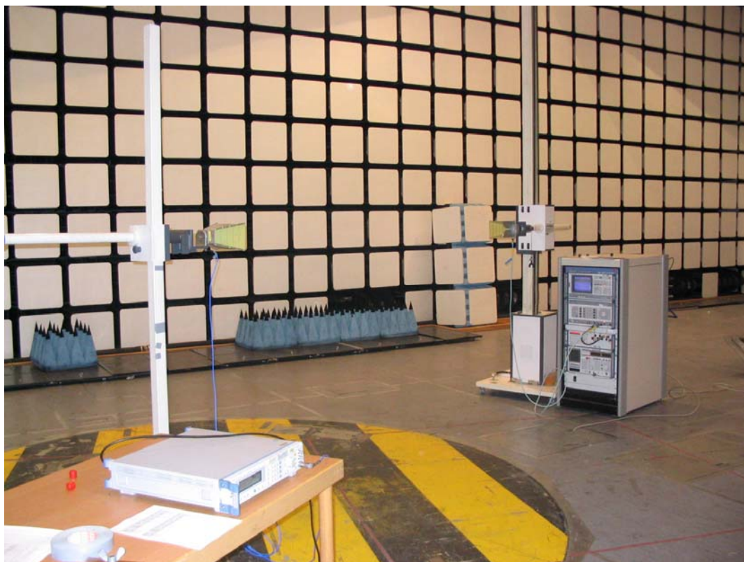
Fig. 55 – Photograph of the anechoic chamber with the test configuration for substitution method.
