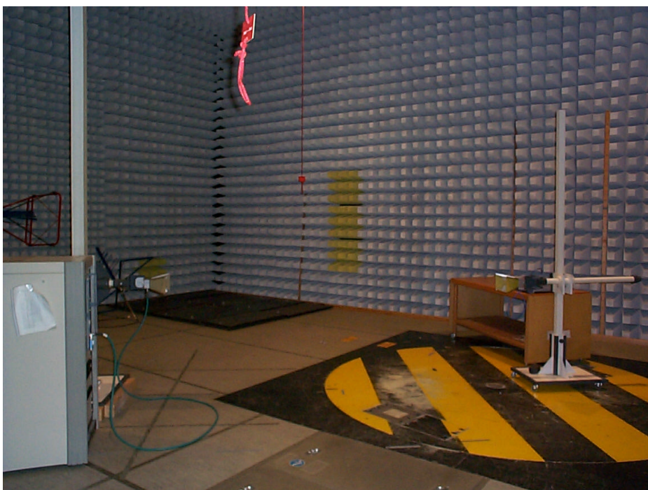
Fig. 92 – Photograph of the anechoic chamber with the test configuration for substitution method
