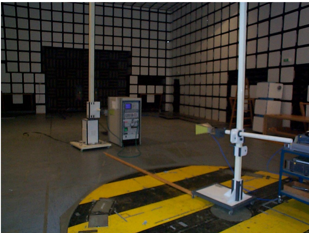
Figure 2: Photograph of the anechoic chamber with the test configuration for substitution method.
