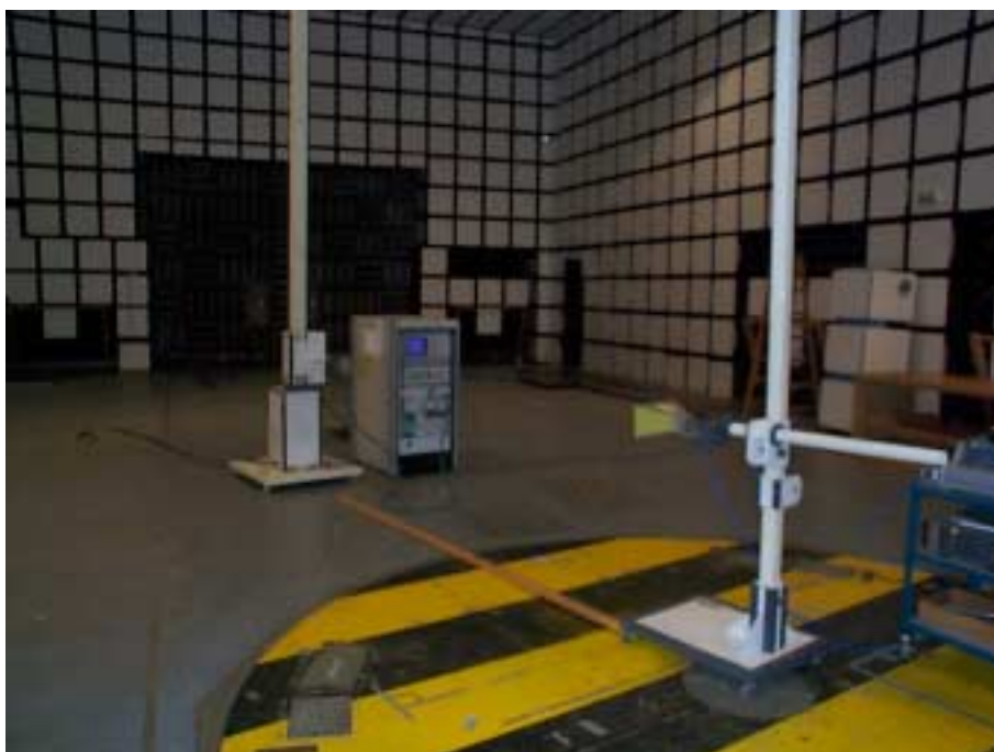
Fig. 27 -- Photograph of the anechoic chamber with the test configuration for substitution method.
