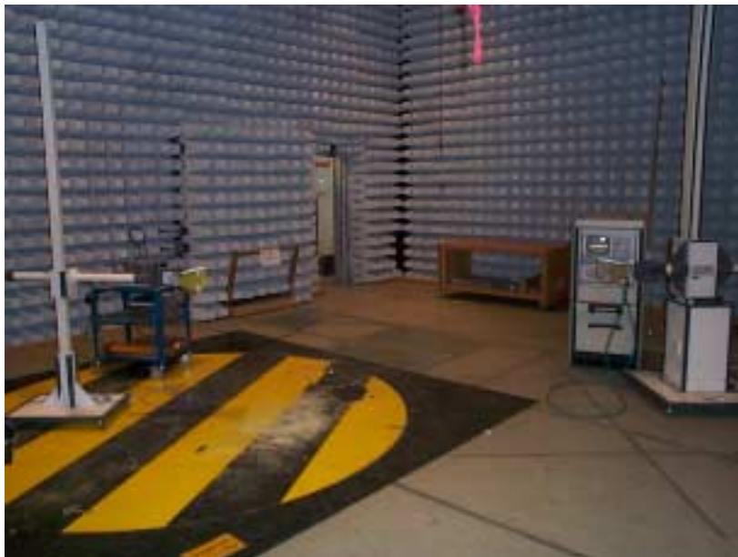
Fig. 35 -- Photograph of the anechoic chamber with the test configuration for substitution method.
