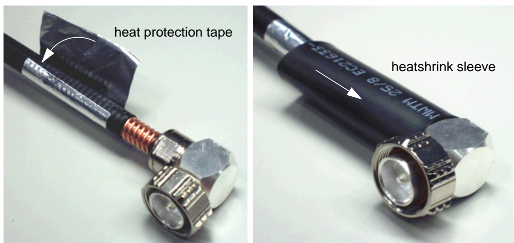
Fig. 2.51 Handling of heat protection tape and shrink sleeve
