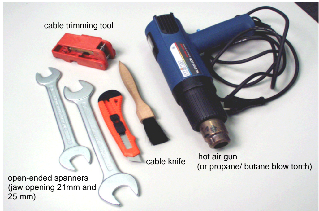
Fig. 2.44 Tools for jumper fabrication
