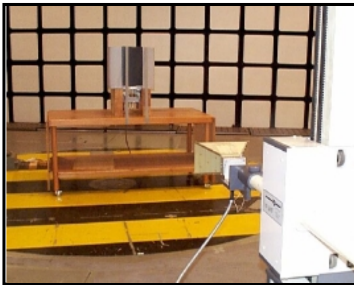
Fig. 26 – Photograph of the anechoic chamber with EUT. The antenna is shown on the right side.
