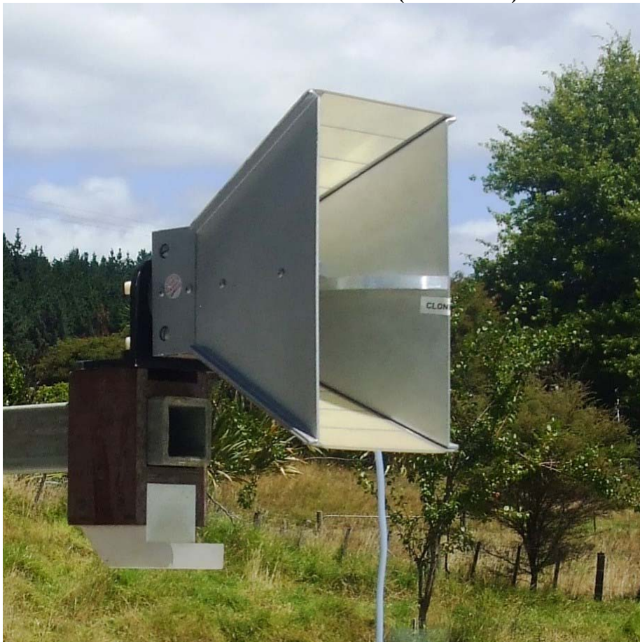
EMCO 3115 Horn Antenna (1 – 18 GHz)
