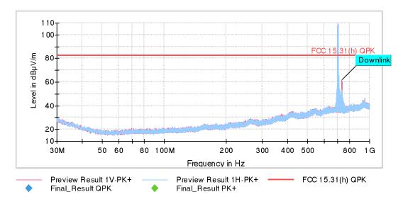
The peak above the limit is the LTE Cat-M1 Band 12 carrier frequency (701.5 MHz).
