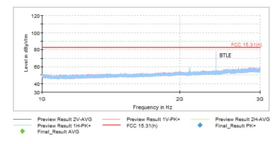
The peak below the limit is the BLE (2M) carrier frequency (2402 MHz).
