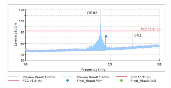
The peak above the limit on the left is the LTE Cat-M1 Band 2 carrier frequency (1880 MHz).
