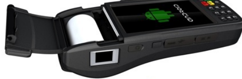
the paperroll cover can be opened when the waterproof cover is open first
