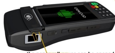
the paperroll cover can be opened when the waterproof cover is open first
