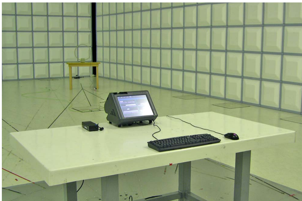
The Front View of Highest Radiated Set-up For EUT (9KHz~30MHz)
