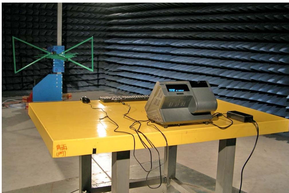
The Back View of Highest Radiated Set-up For EUT (30MHz~1GHz)
