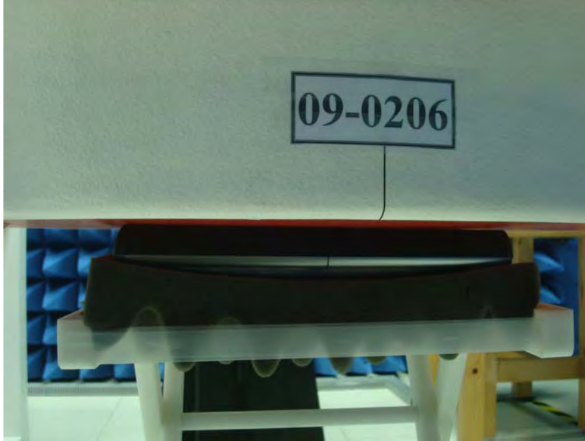
Figure 1. Body SAR Test Setup (Flat Section)
