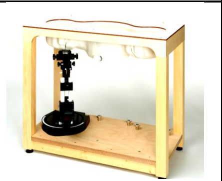
Fig 5.9 Photo of SAM Phantom
