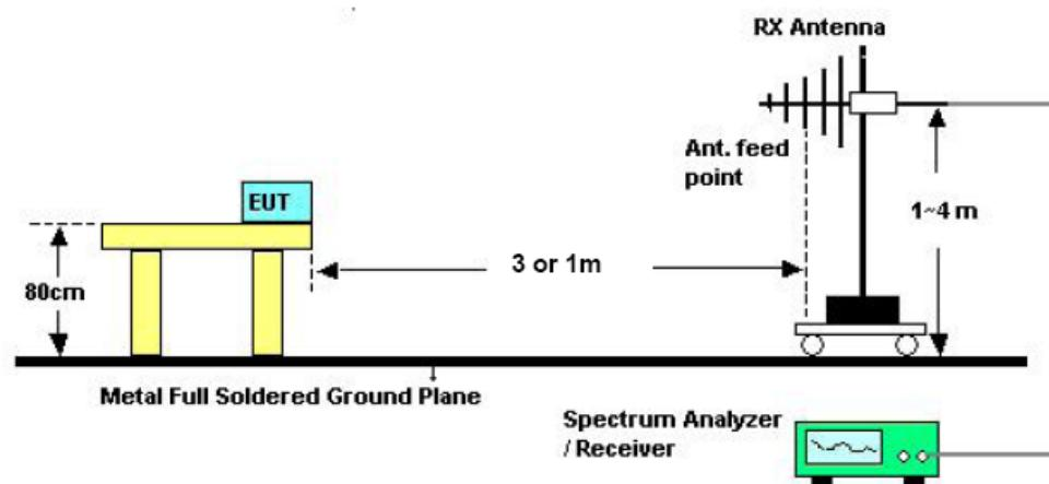
Above 10 GHz shall be extrapolated to the specified distance using an extrapolation factor of 20 dB/decade from 3m to 1m.
