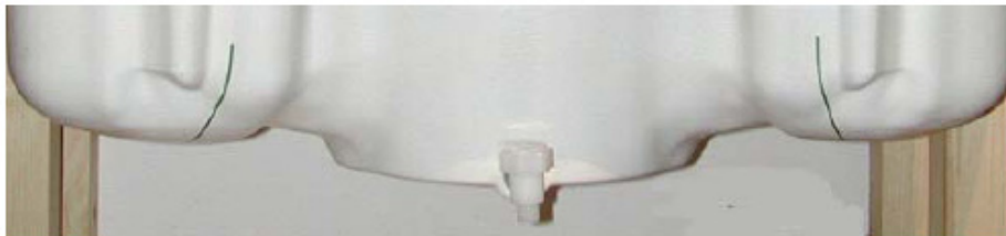
Figure 7.2 SAM Twin Phantom shell
