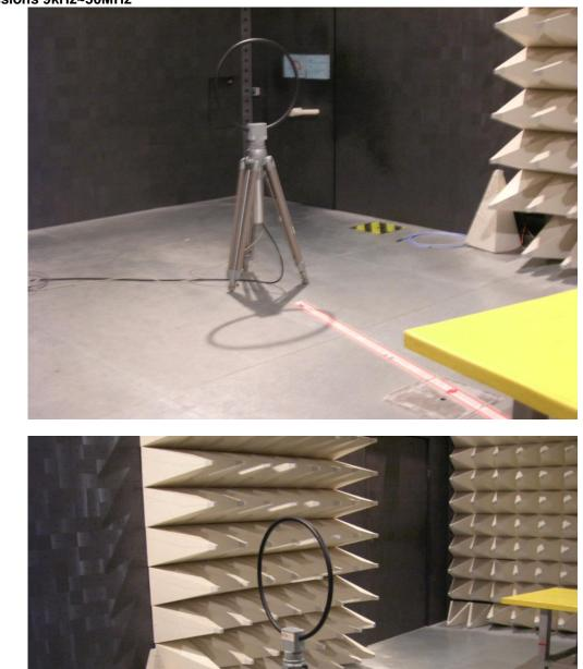
2 Photographs of Radiated Emissions Test Configuration For radiated emissions 9kHz~30MHz
