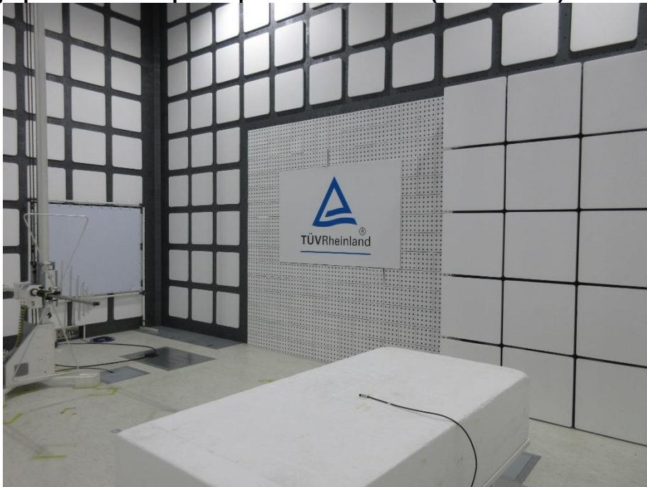
Photograph 4: Test Setup for Spurious Emissions (Back View 2)
