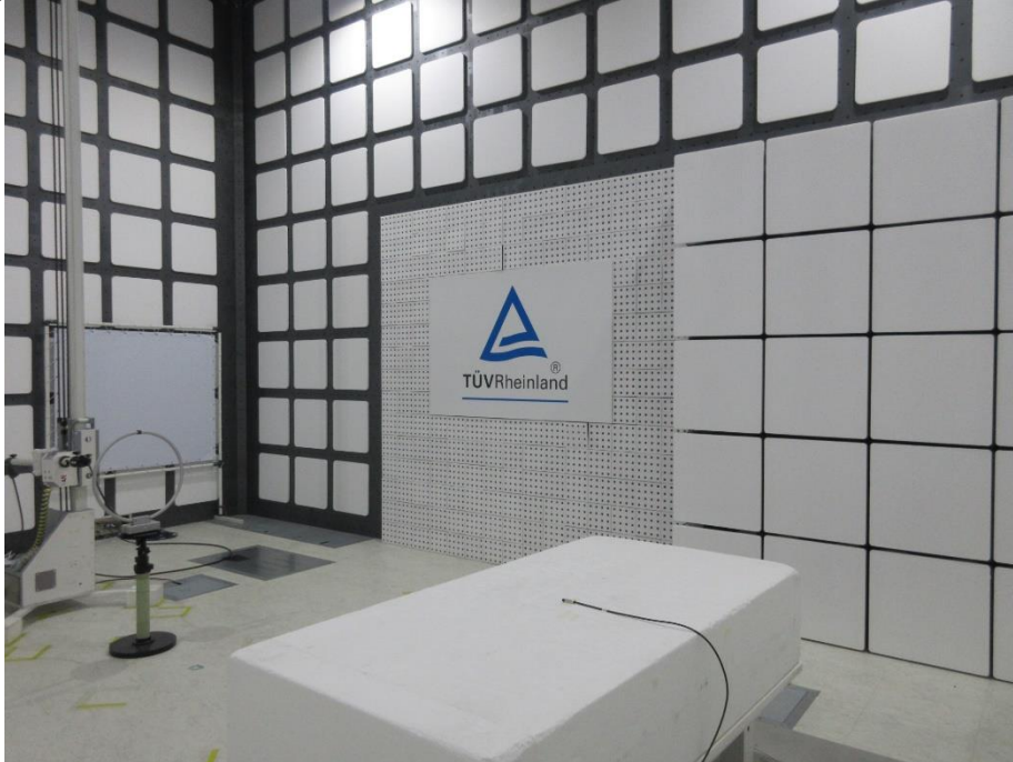
Photograph 3: Test Setup for Spurious Emissions (Back View 1)
