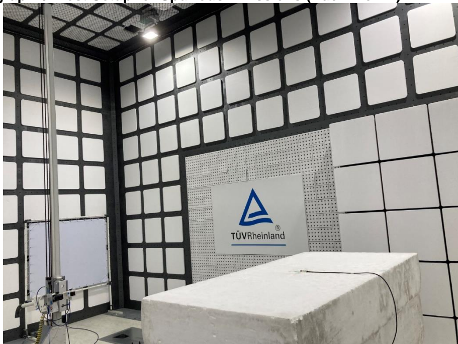
Photograph 6: Test Setup for Spurious Emissions (Back View 4)
