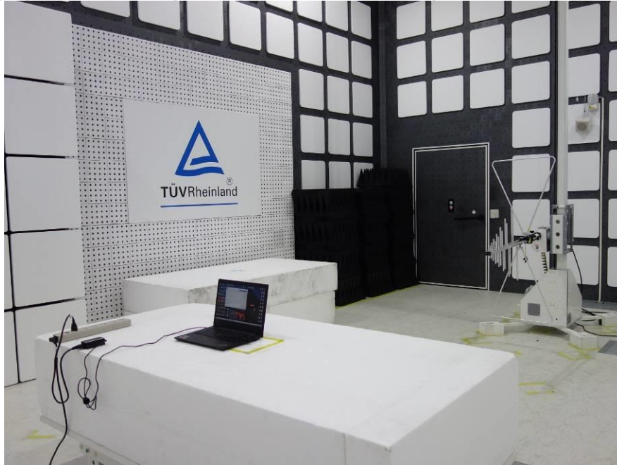
Photograph 4: Test Setup for Spurious Emissions (Back View 2)
