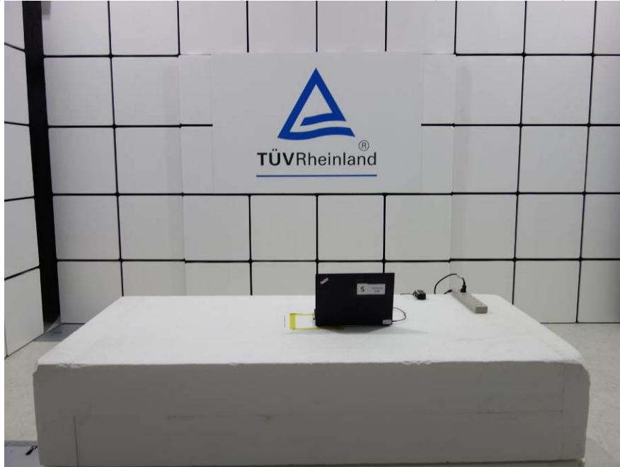
Photograph 1: Test Setup for Spurious Emissions (Front View 1)
