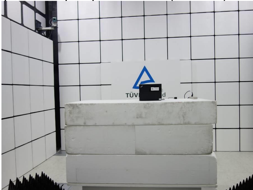
Photograph 2: Test Setup for Spurious Emissions (Front View 2)
