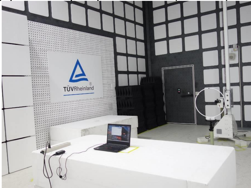
Photograph 4: Test Setup for Spurious Emissions (Back View 2)
