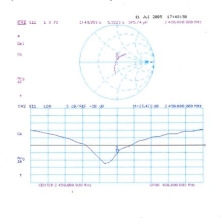
Impedance Measurement Plot for Body TSL
