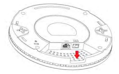
**2.** Connect a router or a PoE switch to the access point's **LAN 1** port using an Ethernet cable.
