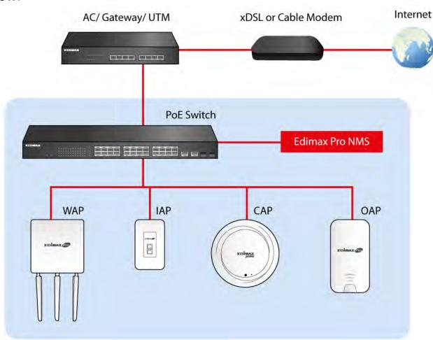
One AP (access point) is designated as the AP Controller (master) and other connected Edimax Pro APs are automatically designated as Managed APs (slaves). Using Edimax Pro NMS you can monitor, configure and manage all Managed APs (up to 16) from the single AP Controller.
