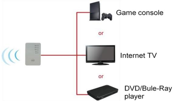
8. Use Ethernet cable to connect it to Ethernet port of your networking device.
