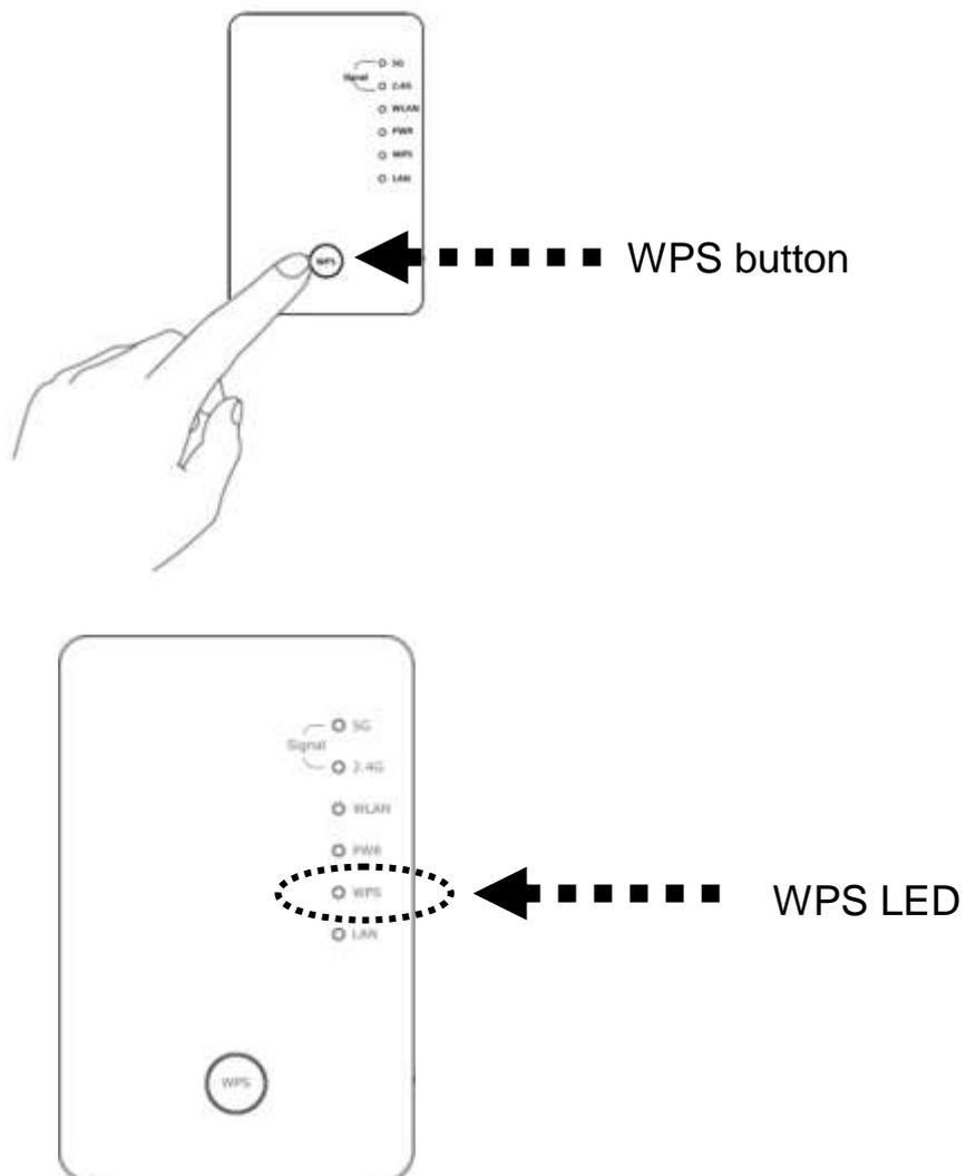
2. Press WPS button on the wireless broadband router or access point you wish to connect within 2 minutes.
