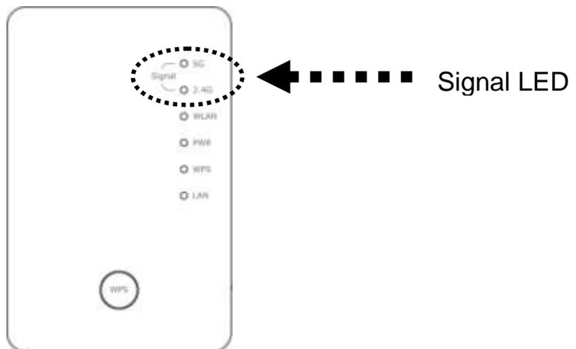
4. ‘**Signal**’ LED in AP mode is Steady light to provide wireless clients the best signal.
