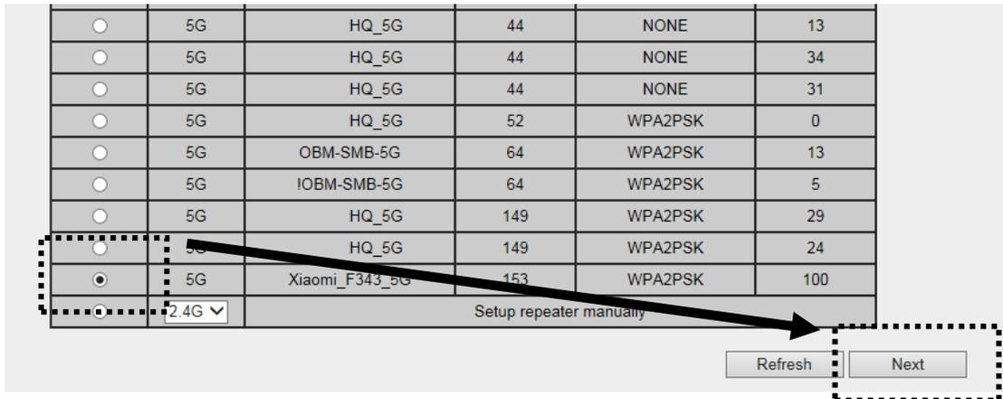
If you want to connect to a hidden access point, you can select **"Setup repeater manually"** to input wireless setting manually.
