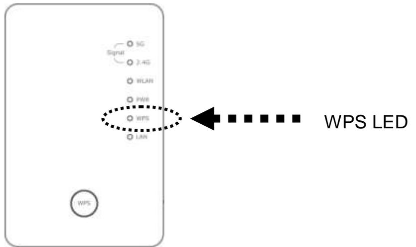
2. Press WPS button on the wireless broadband router or access point you wish to connect within 2 minutes.
