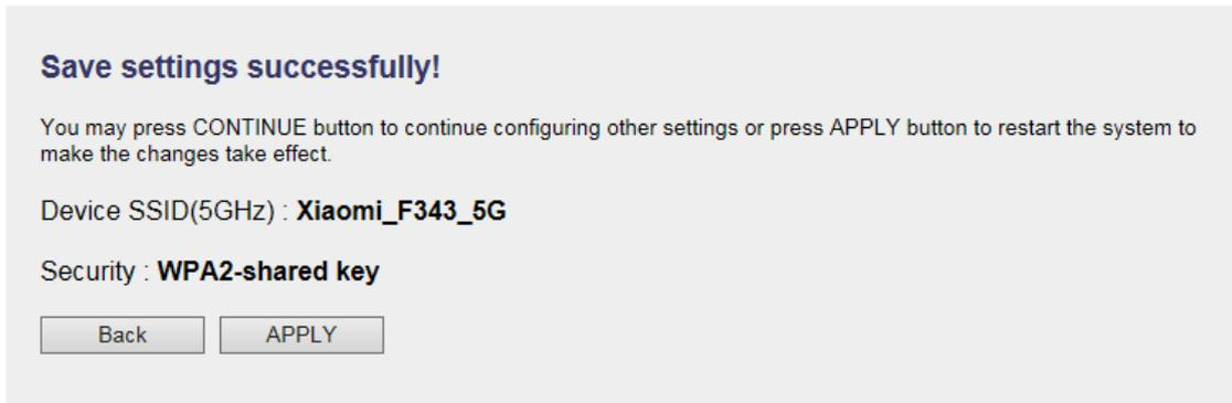
‘Device SSID’ is the SSID of your access point that you selected to connect in previous step, please double confirm all information is correct, if you want to change it, you can press ‘Back’ to select again or press ‘APPLY’ to take this change effect.
