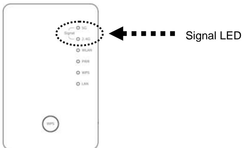
4. Please move repeater to the place you wish to use (a better place will be the center of your house) and insert this repeater into power outlet on the wall, the wireless connection will be established automatically. You can check '*Signal*' LED status to understand signal reception level.
