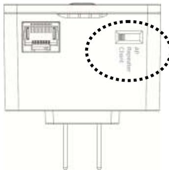
Insert this device into power outlet on the wall. You should see '**Power**' LED light up in few seconds. If not, please check if the power outlet you're using is working.
