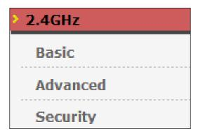
The "2.4GHz" menu allows you to access basic, advanced and security settings for your access point's 2.4GHz wireless networks. You can also enable or disable the access point's 2.4GHz wireless networks.
