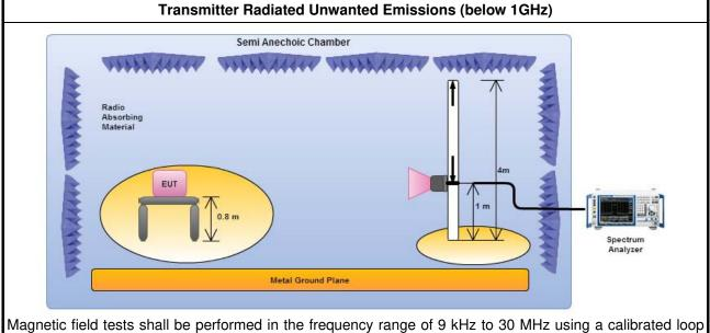
antenna. Electric field tests shall be performed in the frequency range of 30 MHz to 1000 MHz using a calibrated bi-log antenna.
