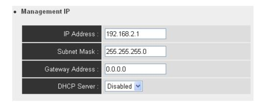
Please input IP address and Subnet Mask in corresponding field, and you can input the IP address of gateway in 'Gateway Address' field, if you need to manage this wireless access point from other network (like Internet).
