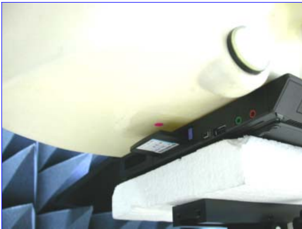
Figure 13. Top (Notebook PC touching SAM Phantom) Distance of the PCMCIA card to the phantom = 1.5 cm The laptop computer was opened in this position.
