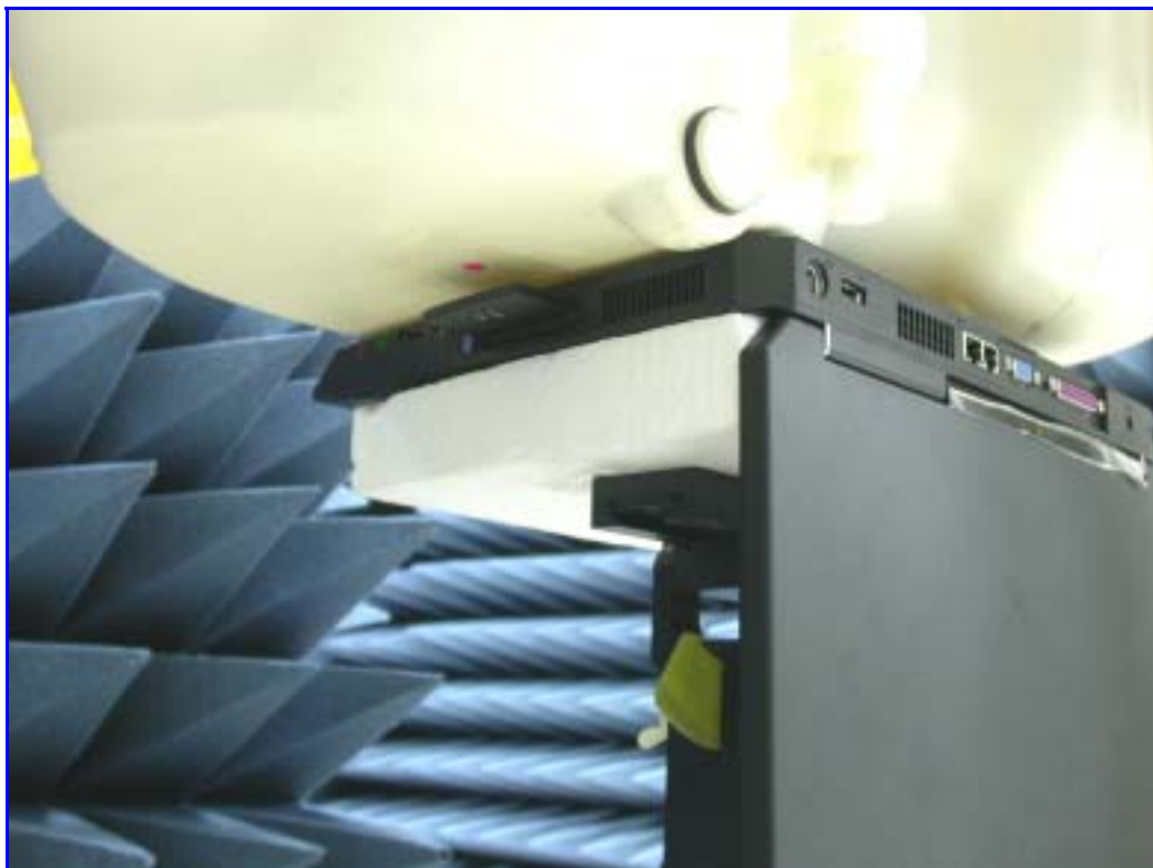
Figure 11. Bottom (Notebook PC touching SAM phantom) Distance of the PCMCIA card to the phantom = 1.1 cm
