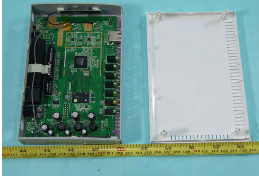
PIFA antenna with USB port
