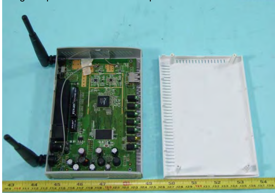
Integral dipole antenna with USB port
