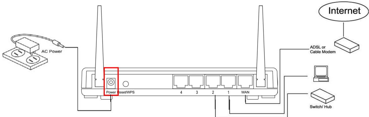
4. Please check all LEDs on the front panel. 'PWR' LED should be steadily on, WAN and LAN LEDs should be on if the computer / network device connected to the respective port of the router is powered on and correctly connected. If PWR LED is not on, or any LED you expected is not on, please recheck the cabling, or jump to '**4-2 Troubleshooting**' for possible reasons and solution.
