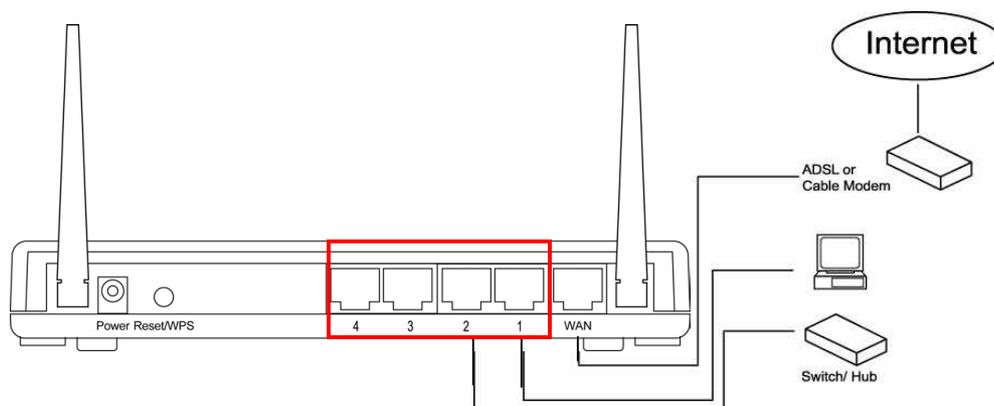
3. Connect the A/C power adapter to the wall socket, and then connect it to the 'Power' socket of the router.
