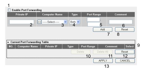
Enable Port Check this box to enable port mapping,
