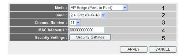
NOTE: Two wireless routers must use the same mode, band, channel number, and security setting!
