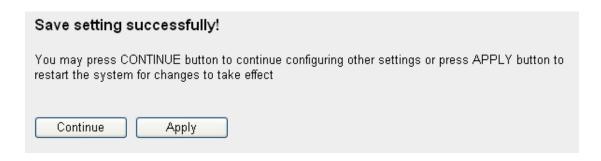
Press 'Continue' to save the settings made and back to web management interface; press 'Apply' to save the settings made and restart the router so the settings will take effect after it reboots.
