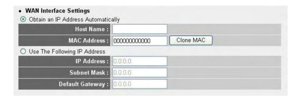
Select the type of how you obtain IP address from your service provider here. You can choose 'Obtain an IP address automatically' (equal to DHCP, please refer to 'Cable Modem' section above), or 'Use the following IP address' (i.e. static IP address).
