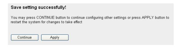
Press 'Continue' to save the settings made and back to web management interface; press 'Apply' to save the settings made and restart the router so
