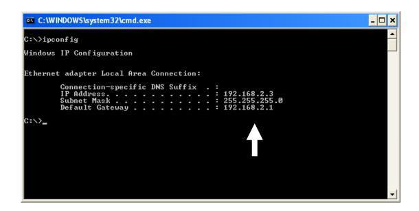
NOTE: If the IP address of Gateway is not displayed, or the address followed by 'IP Address' begins with '169', please recheck network connection between your computer and router, and / or go to the beginning of this chapter, to recheck every step of network setup procedure.
