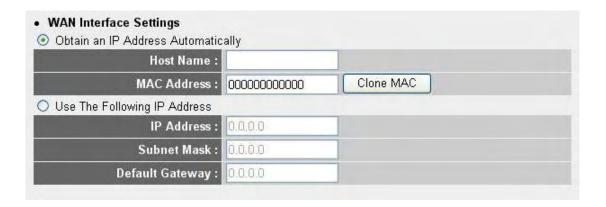
Please select the type of how you obtain IP address from your service provider here. You can choose 'Obtain an IP address automatically' (equal to DHCP, please refer to 'Cable Modem' section above), or 'Use the following IP address' (equal to static IP address, please refer to 'PPPoE xDSL' section above).
