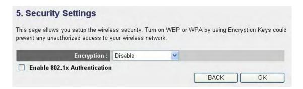
Please choose the Encryption type you're using from the dropdown list of "Encryption". There are three types of Encryption, they are:
