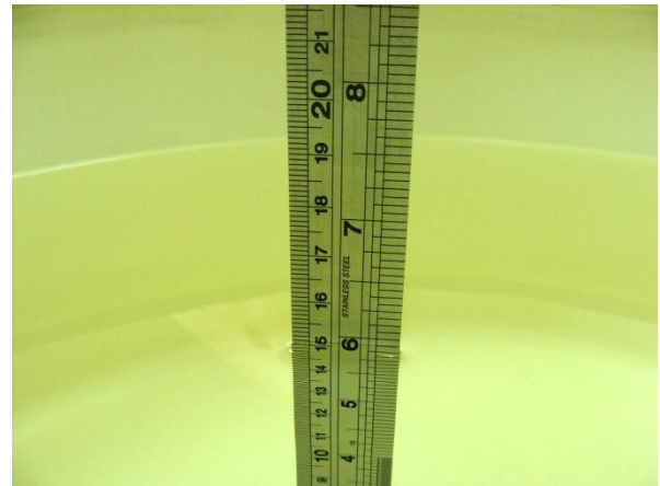
Fig 6.2 Photo of Liquid Height for Body SAR
