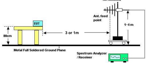
Above 10 GHz shall be extrapolated to the specified distance using an extrapolation factor of 20 dB/decade form 3m to 1m.
