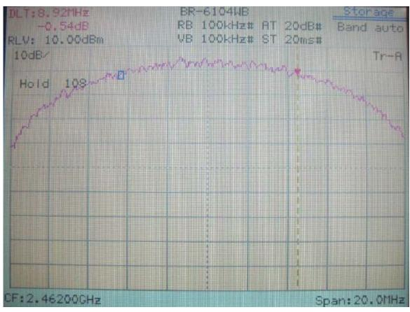
6dB Bandwidth of Channel 11: 8.92MHz (The minimum 6dB BW at least 500kHz)
