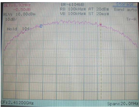
6dB Bandwidth of Channel 1: 8.92MHz (The minimum 6dB BW at least 500kHz)
