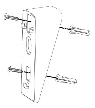
**2.** Attach the rear of the network camera to the mounting stand and tighten into place, as shown below:
