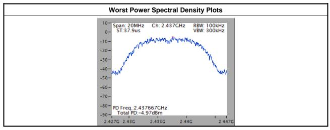
Note: 15.2dBm has been offset for 3kHz data.
