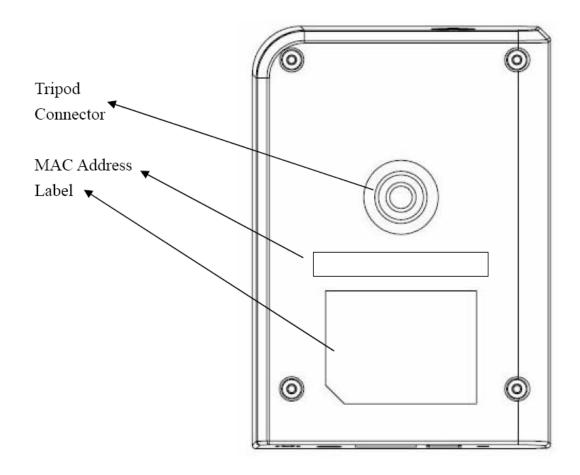
Tripod Connector: Connects to any standard tripod / camera wall holder. MAC Address Label: Shows the MAC address of this IP camera. Useful when you can't locate the camera on the network.
