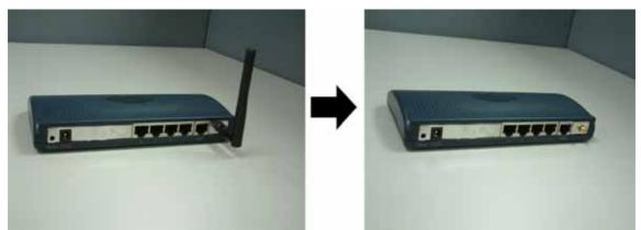
2) Connect the signal booster to the certified wireless router using the included color coded connector cable. Connect the gray end to the input connector on the left side of the signal booster, Connect the white end to the antenna connector on the antenna connector on the certified wireless router.
