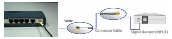
3) After you have connected the signal booster to the certified wireless router, take the antenna included in the package and connect it to the antenna connector on the signal booster. Screw the antenna base in clockwise until the antenna is firmly connected to the booster.
